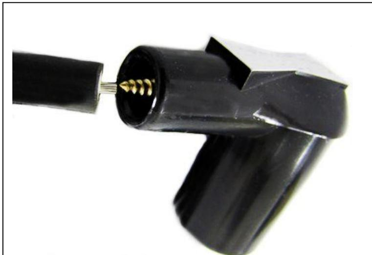
*Whereas a resistor spark plug cap alone is OK, the combination of a resistor cap with a resistor plug and a resistor type lead will seriously reduce the spark at the tip of the plug.*
