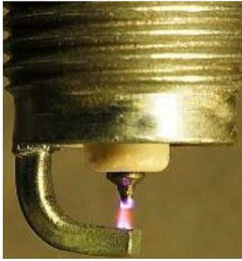
←The spark jumps the gap between the electrodes
