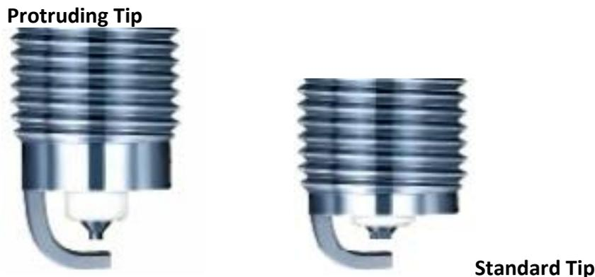
As can be seen from the two photographs above, the protruding tip type spark plug has much more of the ceramic insulator protruding below the threads. Also the area below the plug threads and the central live electrode are both longer than on a standard plug.
