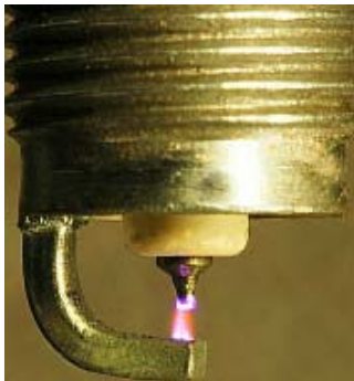
This is how the spark plug works inside the engine
